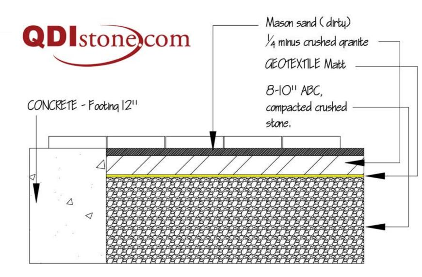
**CONCRETE FOOTER** at perimeter area to prevent lateral movement. 12" depth by 8" avg.
